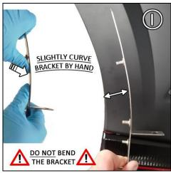
**FIGURE J** To nest the inner rear section of the mounting Bracket close to the liner after it's installed, gently curve the inner rear section of the bracket by hand as shown in Figure J. **DO NOT CURVE THE BRACKET AGGRESSIVELY BEYOND THE LINER**. Make slight adjustments. **FIGURE K & L** Position Bracket sideways as shown, then rotate 90 degrees to install the rear tab between the fender liner and bumper skin.
